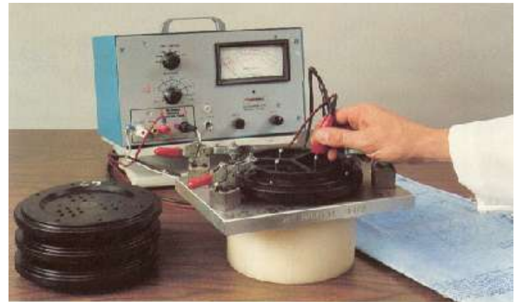
ABOVE: Using a Hipotronics high-voltage megohmmeter, a product's insulation resistance is measured in accordance with method 302 pf MIL-STD-202.
