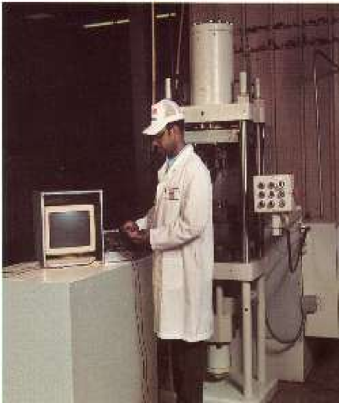
The 75-ton Stokes press has programmable control drive, heat controls, CRT, and data collection.
