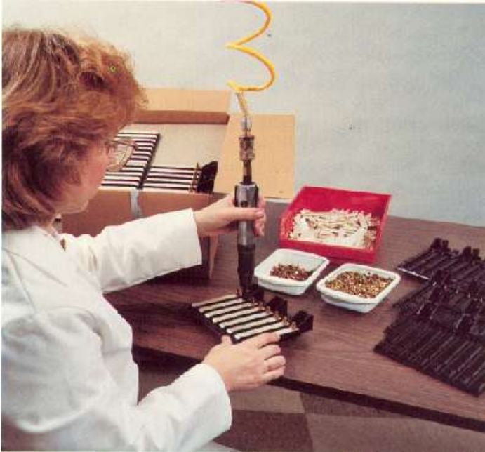
After molding, a secondary contact is assembled and supplied in KANBAN releases approximately every 10 days.
