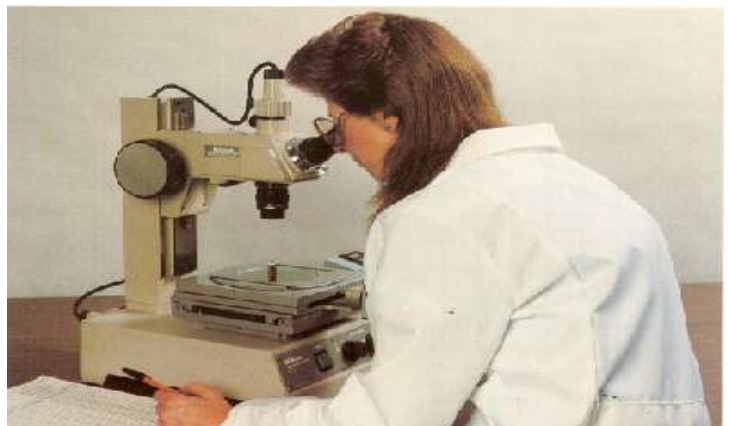
BELOW: The Nikon Measurescope affords us versatility and accuracy when measurement data is required on very small parts.
