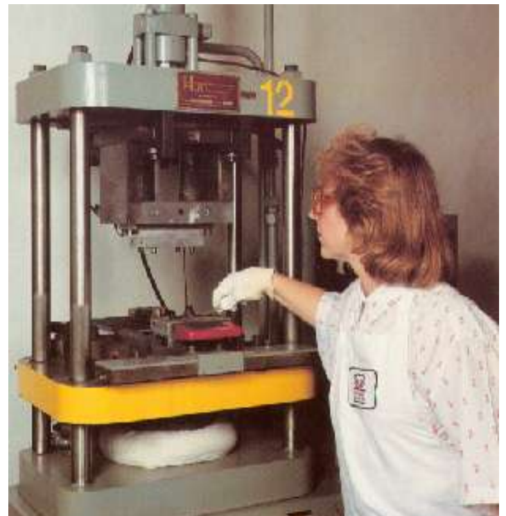
Insert molding is one of our specialties. The delicate touch of an experienced operator is critical in this 25-ton transfer molding press.
