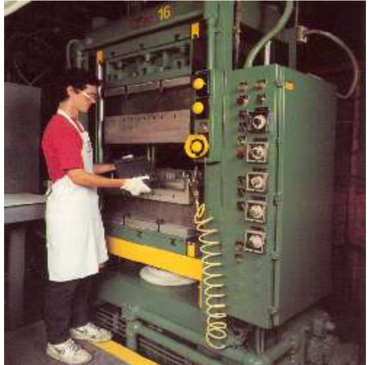
A 200-ton compression molding press run by a meticulous operator and backed by rigorous maintenance program.
