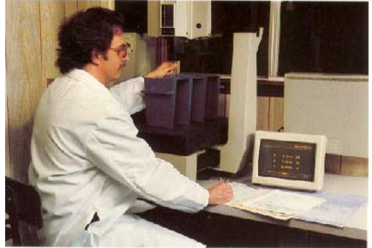
Precise, consistent and fast first-piece inspection with the Brown & Sharpe Microval Coordinate Measuring Machine (CMM) allows PENN to move quickly from verification to production.
